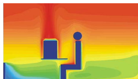
Temperature distribution in the symmetry plane of a room with displacement ventilation.
